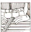
Be sure that: The LEVAKNIFE is clean, plug it into the correct voltage (220V) electricity supply and let it warm up.
