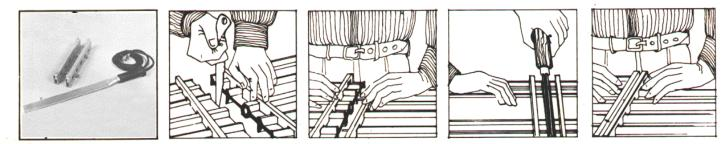
Be sure that: The LEVAKNIFE is clean, plug it into the correct voltage (220V) electricity supply and let it warm up.
