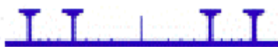
External Plain Web LEVAJOINT Waterstops for use in construction and Construction & Contraction joints
